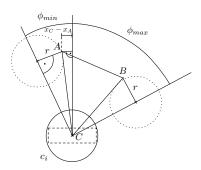
Figure 5: Computing the minimum and maximum angles  $\phi_{\min}$  and  $\phi_{\max}$  for intersecting  $c_i$  with a line.  $\phi_{\min} = -\arcsin((x_C - x_A)/||\overline{AC}||) - \arcsin(r/||\overline{AC}||)$ .
